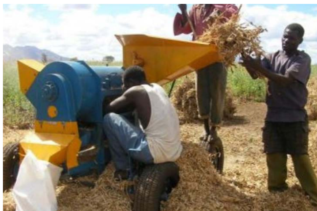
Figure 44: Soya bean threshing by mechanised thresher, Lango, Uganda
