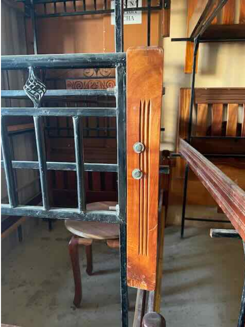
Melia volkensii bed produced by Zombe, in Kitui. Some yellow sapwood is visible: while undesirable, it is rather common across the available supply.
