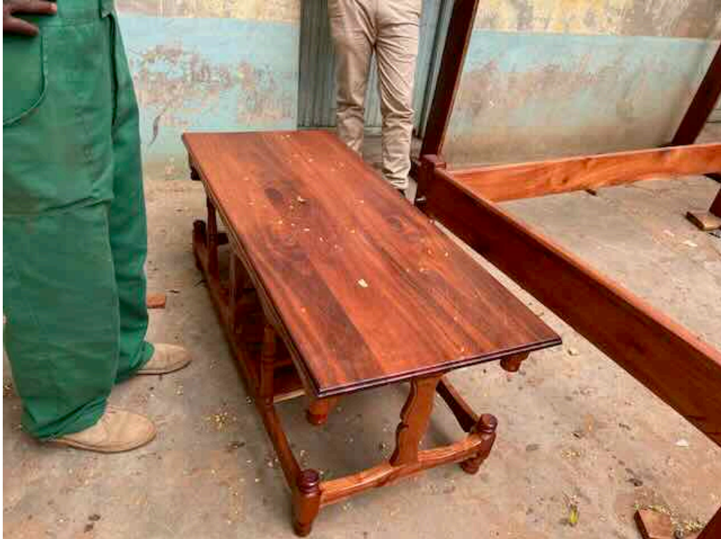
Melia volkensii furniture produced by a small woodworking workshop in Mutomo. Knots from poor silviculture can be observed.
